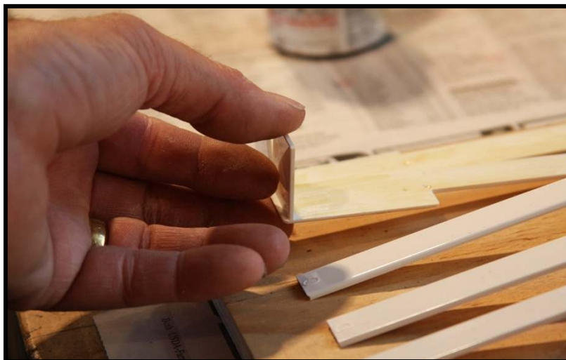
Photo 19: Place glued keytops on pallet with top surface.
