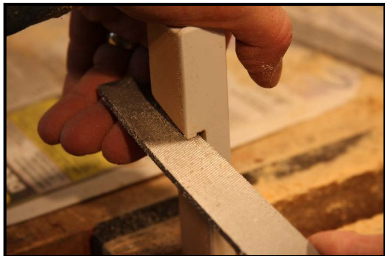
Photo 28: Finishing the notch.
