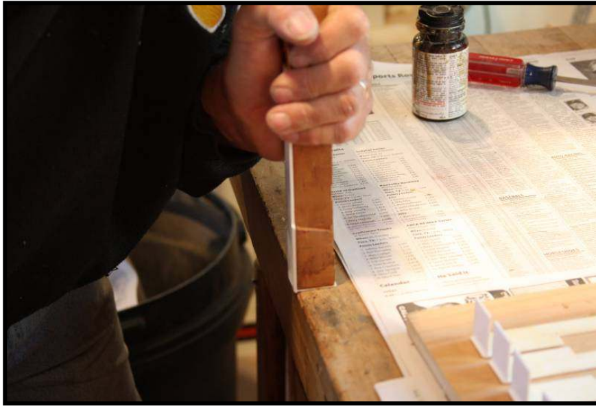
Photo 21: Pushing down on the front to create the bond.
