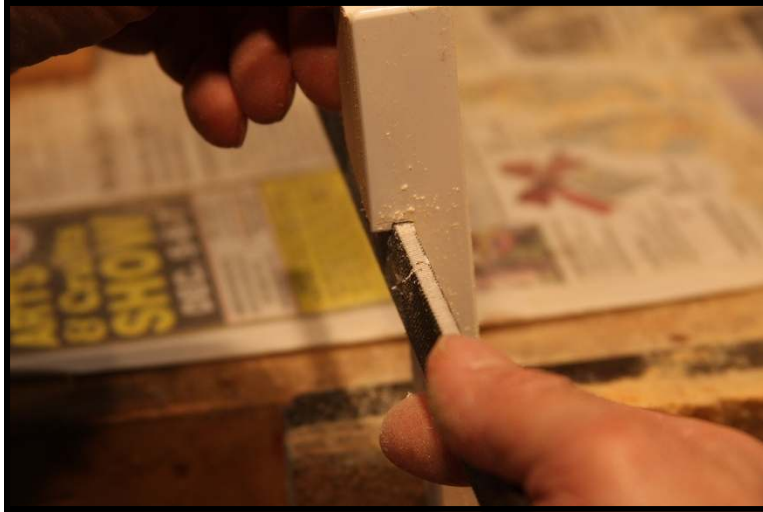
Photo 27: Cutting the notch.
