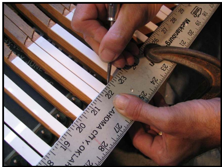
Photo 25: Making a scratch line.
