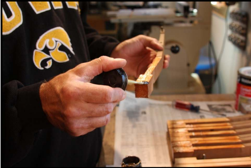
Photo 14: Applying second coat of contact cement.
