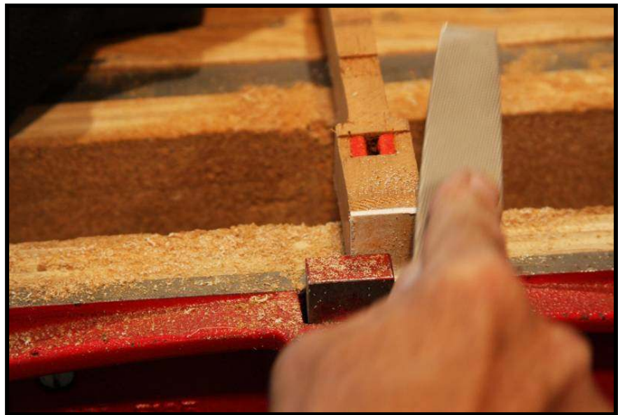
Photo 22: Filing the front of the key down flush.
