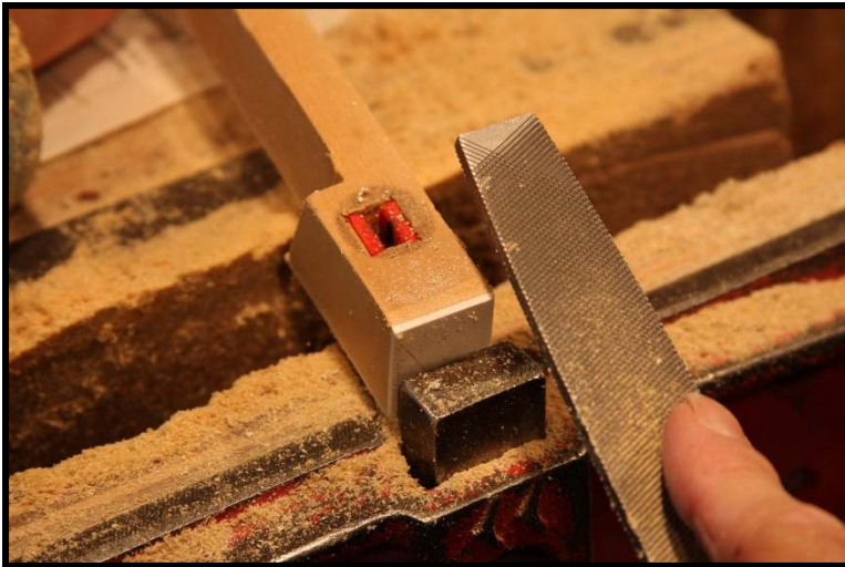
Photo 30: Finishing the bottom of the keyfront.
